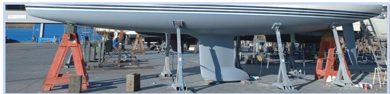
Figure 5. A process of applying an anti-osmosis protector to the entire surface without missing areas.
